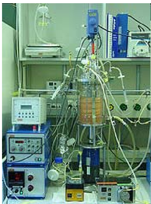
Figura 1.2. Reactor tipo air-lift
