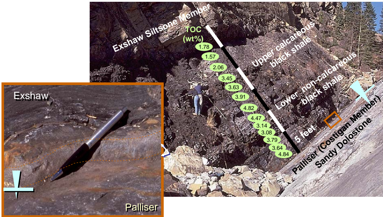
Figure 5b - Example of organic-richness vertical profile and flooding contact in a relatively proximal setting, Exshaw type section, Jura Creek, Alberta, Canada. The flooding surface is marked by the light blue symbol (see inset for detail of this contact), and various parasequence packages are indicated by the breaks in the weathering profile and the TOC vertical variability. A correlative surface and TOC profile are shown in Figure 15.
