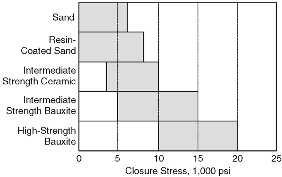
Fig. 4—The recommendations of proppant type based on closure stress the proppant will be subjected to during the life of the well. Taken from Economides et al. (1998).
