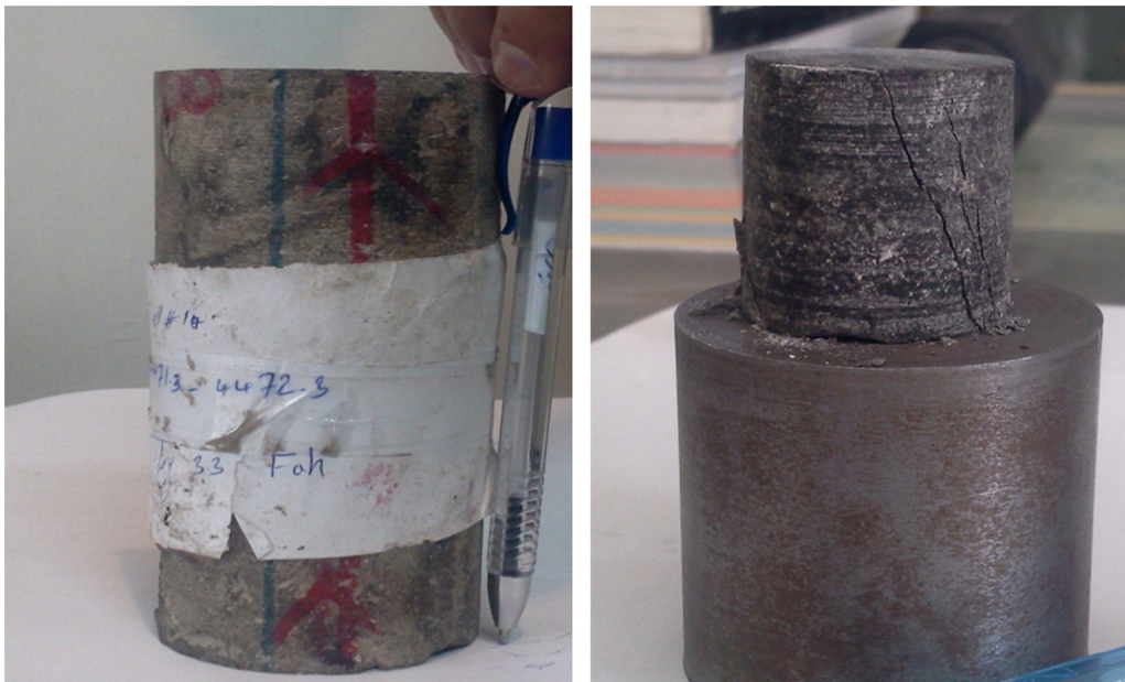
Fig. 4. View of core sample used for UCS test (left) and sample view after the test (right).
