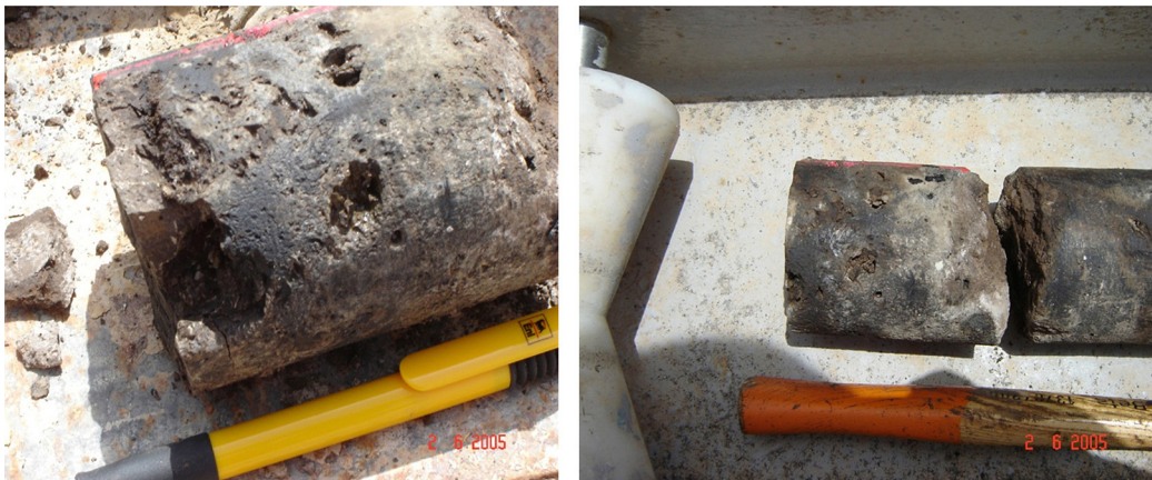
Fig. 2. View of bulk sample from Well B used to acquire plugs for rock mechanical tests.
