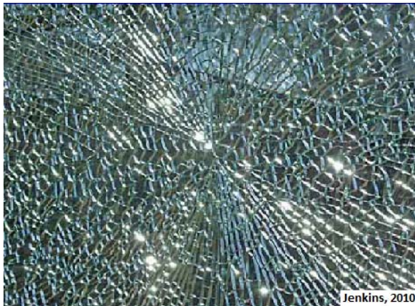
Figure 3 Network or complex fracturing in many shales are envisioned to be similar to that in shattered glass, forming a series of flow paths reaching out a few hundred feet from the wellbore as confirmed by micro-seismic monitoring of the fracture treatments.
