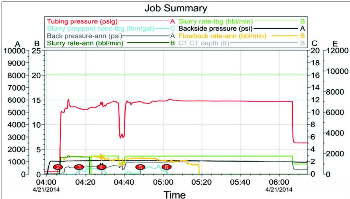
Fig. 17—First stage hydrajetting perforations.
